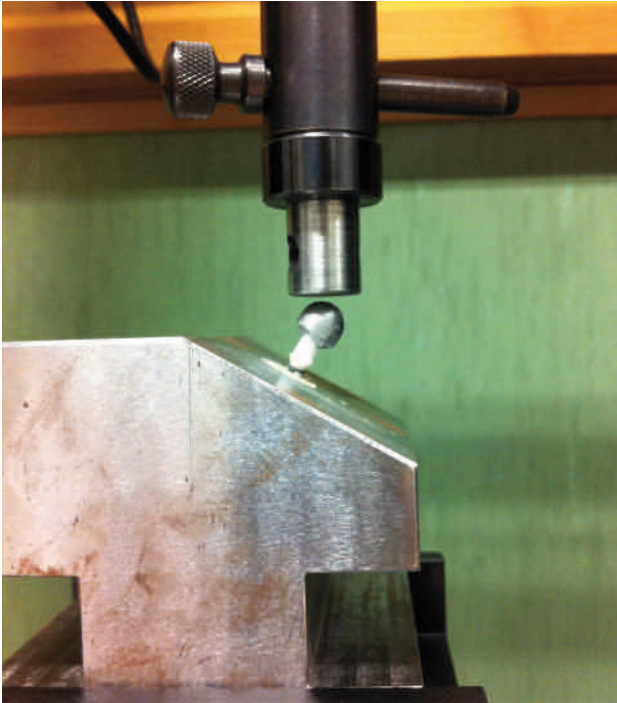
Figure 2. Static strength testing assembly.
